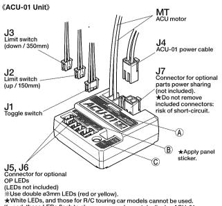
If used, these LEDs flash to show errors and remotely display ACU-01
